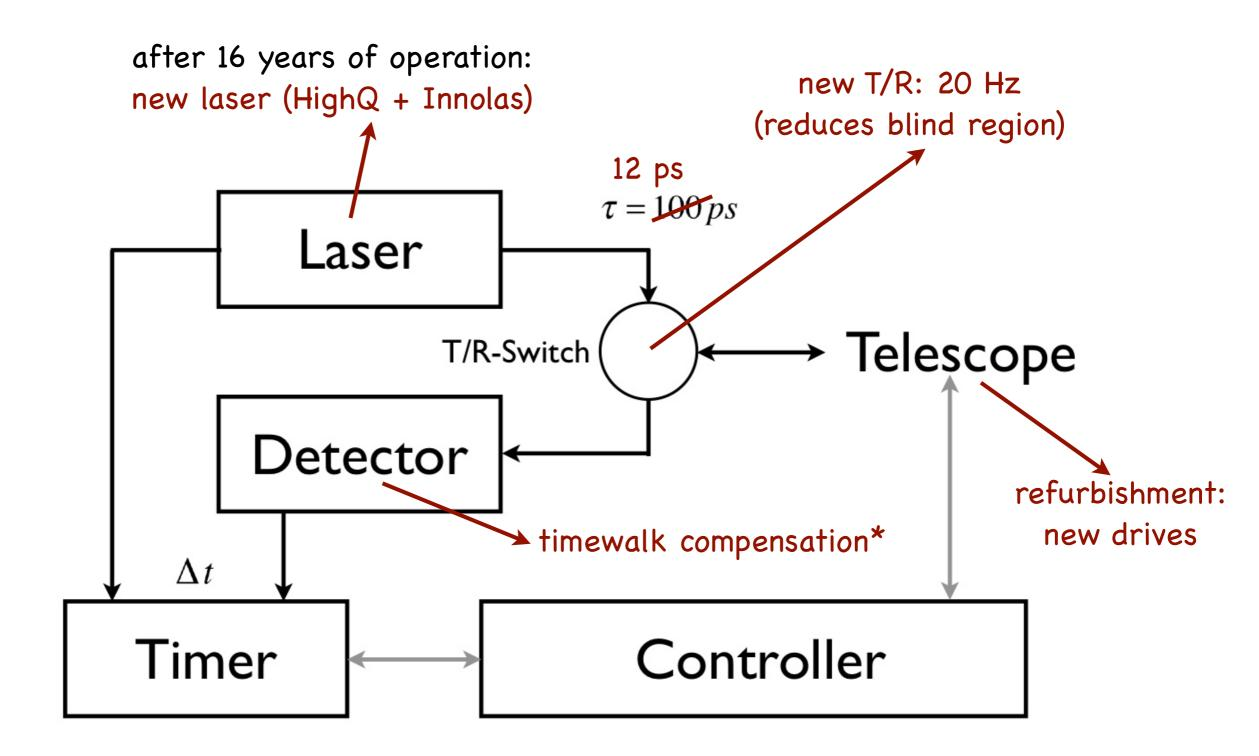
new control system: more autonomous functions, satellite interleaving, improved timer
