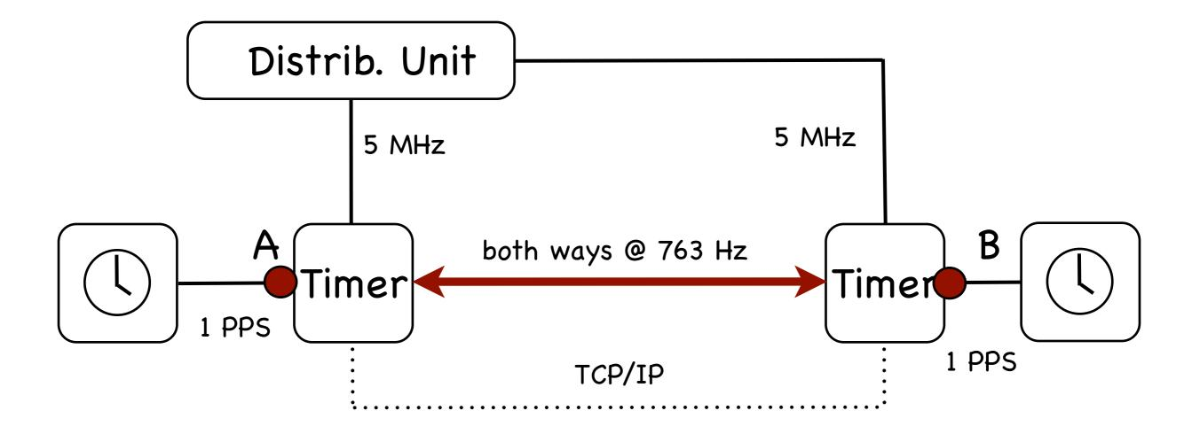
Measurement returns Offset between A and B It also returns the variation in the length of the cable
